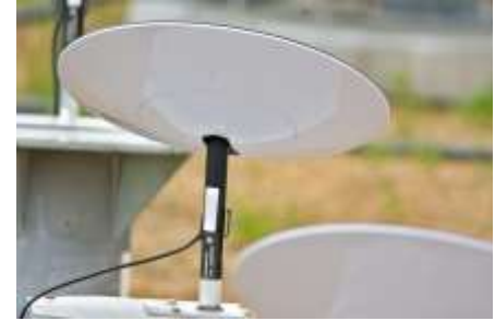
Spacelink Phased Array User Terminal
